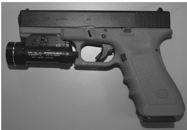
Figure 4.35 (See color insert.) The Glock 22P. The 22P is an inert training aid used to familiarize the user with the pistol without the risk of handling a firearm that could become loaded. The pistol accepts a magazine, and the trigger is fully functional, but the barrel is solid. The red frame is meant to alert the user that this example is inert. (Image from author's collection.)
